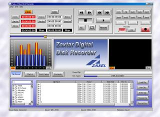
ZAXTAR has internal SATA Disks which have been configured to RAID 50 for storing video and audio, therefore, even when a disk fails, the data will not be lost. Video is captured into AVI files. DPX files can be played back in real time to output RGB video or YUV video.
